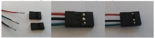
The 3 pin plug shown above (middle) is suitable for ramps, the four pin (right) is setup for Duet wifi/ethernet. Make sure the crimp locks into place in the plug housing, if not rotate it and re-insert it. Check your controller board's documentation carefully!
